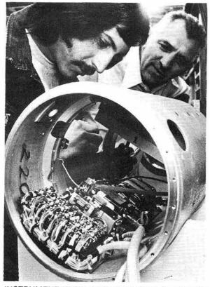
INSTRUMENTATION payload package for rockets launched from the Arctic is assembled by Dennis Armijo, left, and Ted Krein (both 1253). Each of the two rockets fired carried the same type of instrumentation for studying the earth's magnetosphere.
